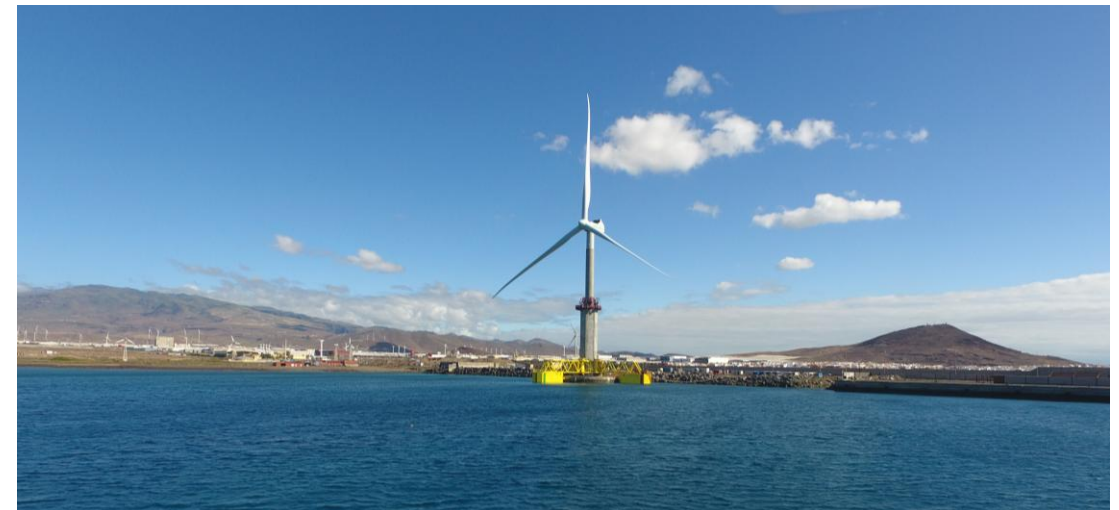
TIM platform coupled to the ELISA GBS substructure prior to tow-out
