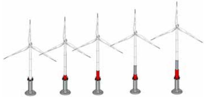
Figure 27: Tower lifting process
