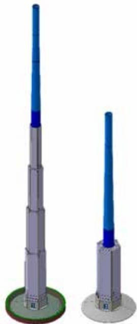
Figure 3: General views of the tower in folded position (before lifting) and unfolded position
