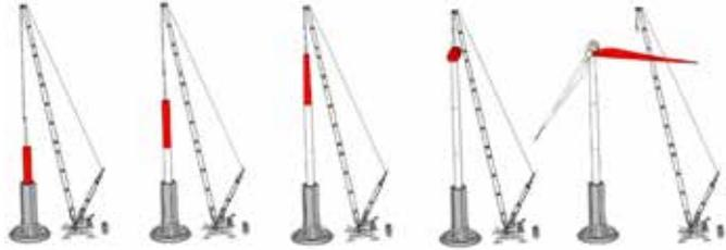
Figure 23: Upper steel tower, rotor and nacelle assembly
