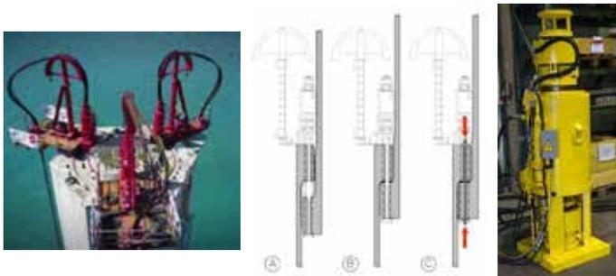
Figure 24, 25 and 26: Stand-jack positioning
